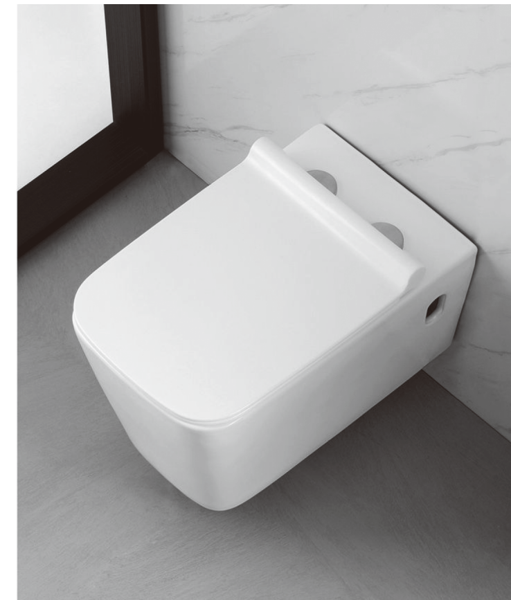
T3201 WALL-HUNG TOILET Size: 560x360x360mm Washdown/P-trap P-trap: 180mm Roughing-in
