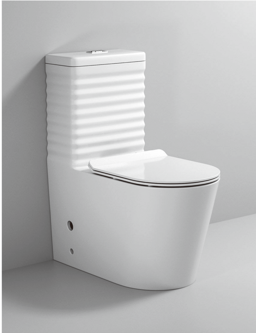
T2126 WASHDOWN ONE-PIECE TOILET Size: 680x370x800mm S-trap : 250mm Roughing-in P-trap : 180mm Roughing-in
